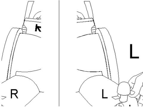
Now press the safety caps from above, making sure that they are attached to the correct sides (engraved right and left).
