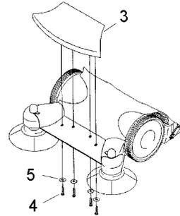
Loosen the four plastic screws (4) on the underside of the dust spoiler (3) and place the screws with the plain washer (5) on the ground.
