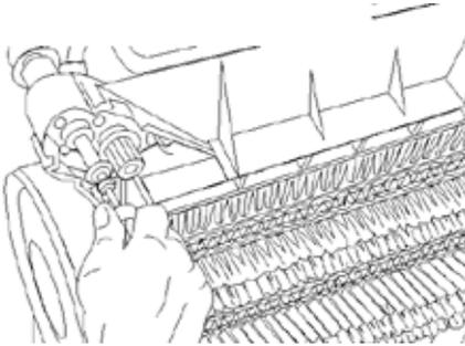
Fold back the handle on the machine. Now put the sweeper upside down on the ground and, remove the screw from the brass axle of the inlet brush.
