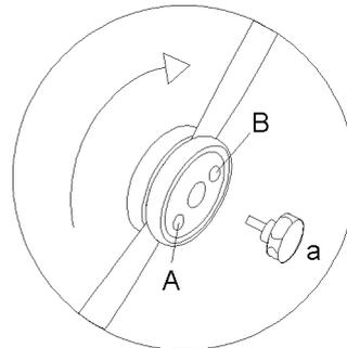
To release strain on the bristles of the sweeping rollers and to save space in storage, you can unscrew the star screws (a) on the left and right of the push bar, fold the bar forwards into the parking position and replace the screw in hole B. The machine can now be stored vertically and requires less space. The container does not need to be emptied to do this.
