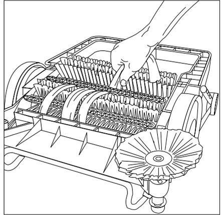
In the event of heavy soiling, grasp the dust filters (left and right) behind the cassette using the screw driver, lift them out completely and either clean the filter or replace it.
