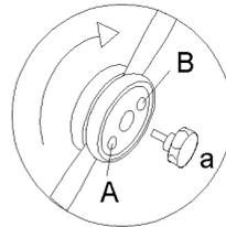
Fix the push bar into the work position in hole (A) using the star screws provided (a).
