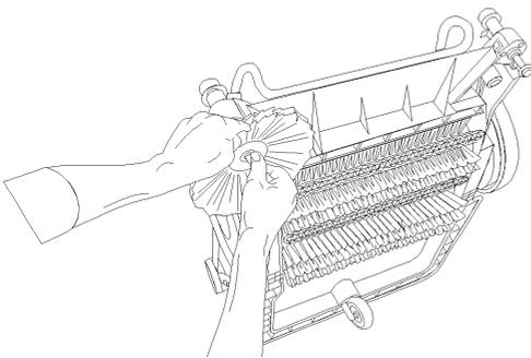
First place washer no. 72 on side brush no. 74 above the ball bearing and place both on bearing bolt A. Tighten the screw with safety washers no. 76 and no. 77 into the bolt.
