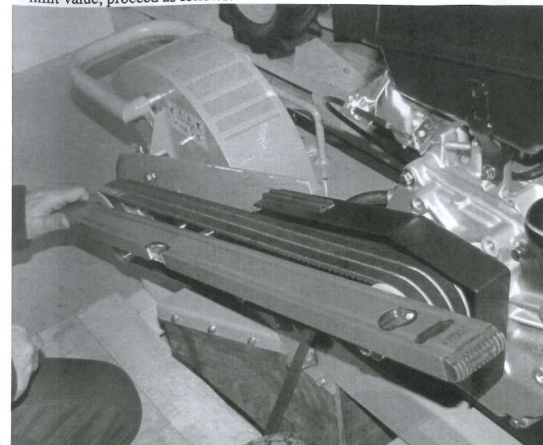
Alignment setting on the engine pulley
