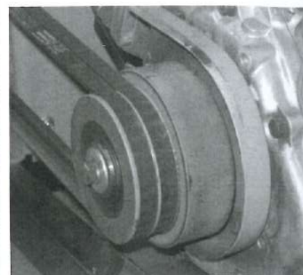
Belt gearing – SWC model with starting clutch
