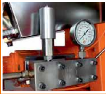
Stainless steel pump-head. Integrated cooling for plunger-seals.
